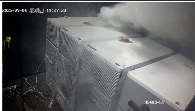
Figure 2.29: During 5 th cell (cell 7) venting (Local Time in 19:27)
