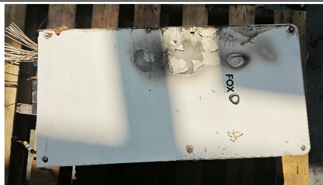
Figure 2.51: Top view of Initiating module after test
