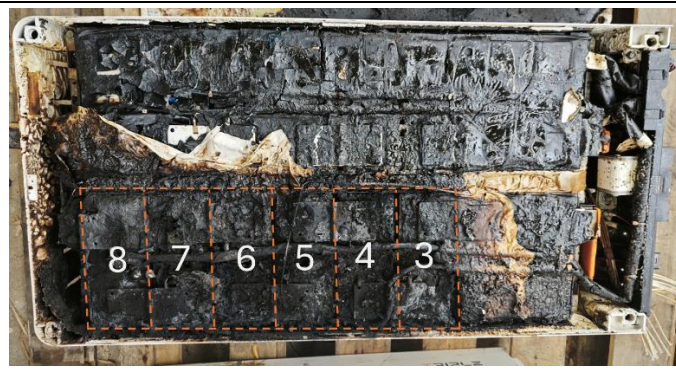
Figure 2.52: Thermal runaway cells
