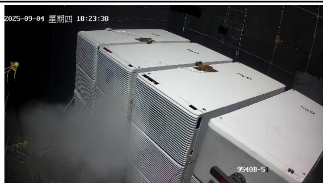
Figure 2.22: During 1 st cell (cell 5) thermal runaway (Local Time in 18:23)
