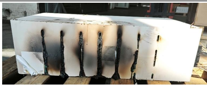
Figure 2.50: Left view of Initiating module after test
