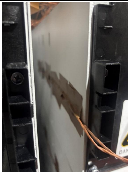
Figure 2.14: Thermocouples on Column C
