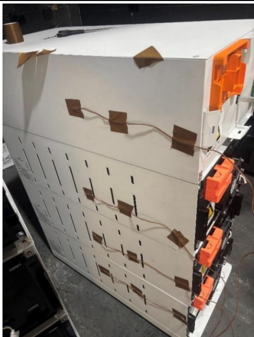
Figure 2.13: Thermocouples on Column D
