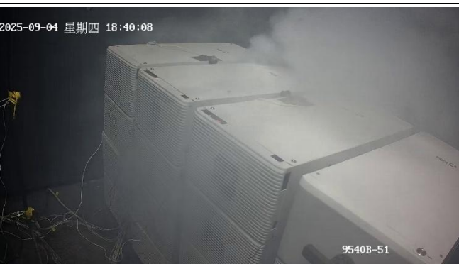
Figure 2.27: During 4 th cell (cell 3) venting (Local Time in 18:40)
