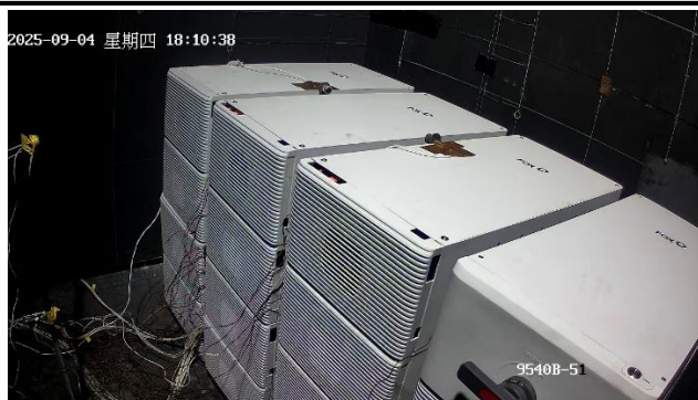
Figure 2.21: During 1 st cell (cell 5) venting (Local Time in 18:10)
